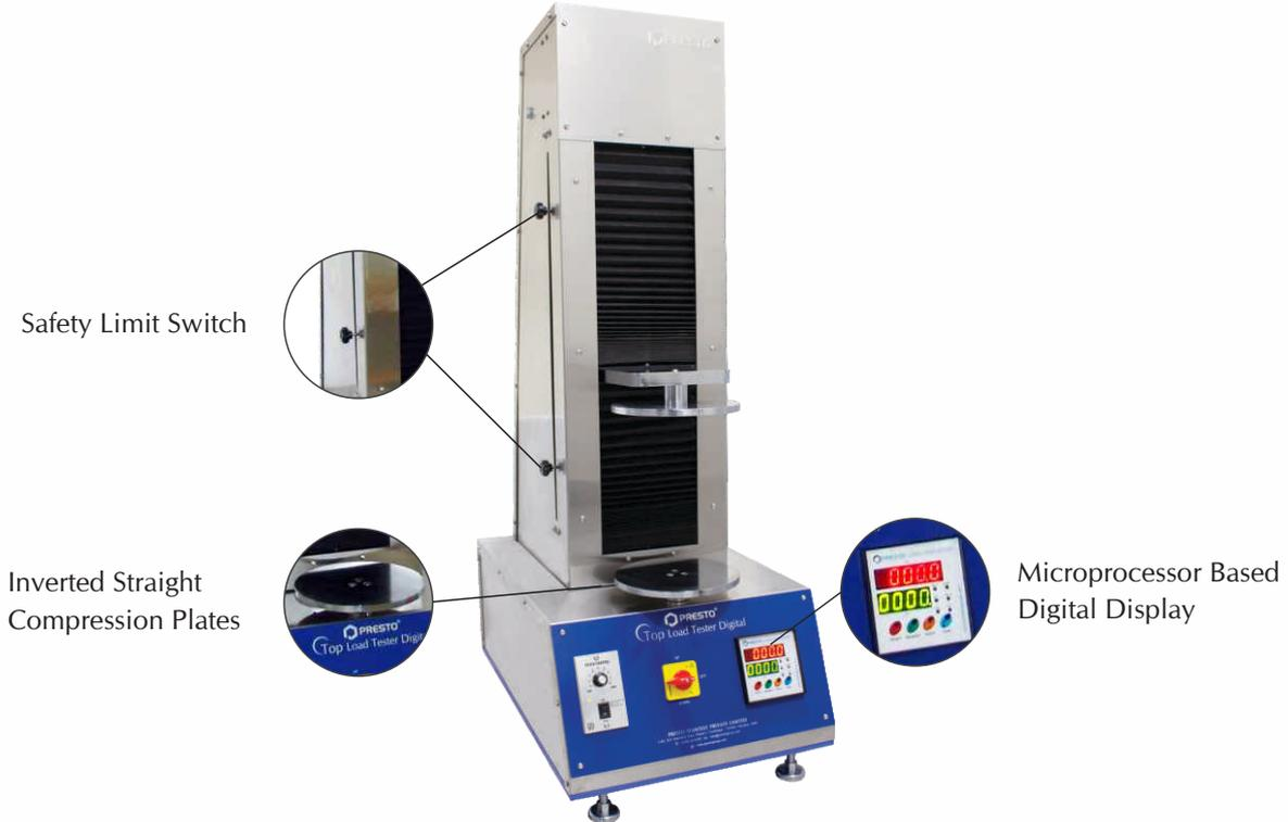
Top - load testing (also known as 'column-crush' and 'axial force resistance') is performed mainly on blow moulded, the reformed or injection moulded plastic containers. It measures the compressive strength of such containers to ensure they do not deform or break when subjected to axial forces during the processes of filling, closure, storage and transport.
